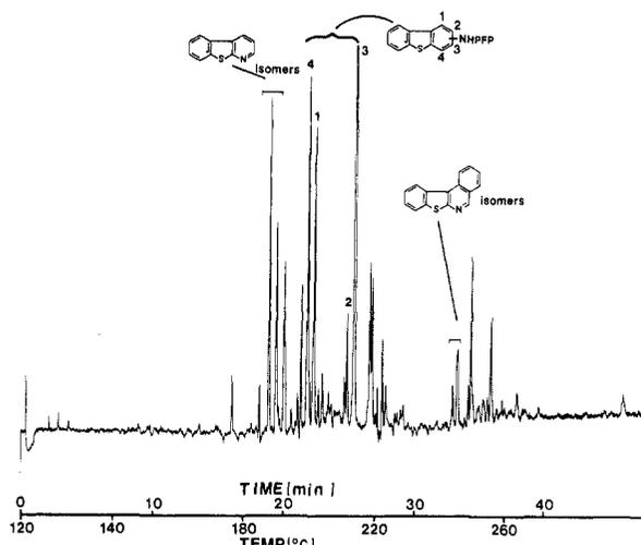
Figure 2. FPD chromatogram of the PFP-derivatized SRC II HD A-3 fraction. Conditions are given in Figure 1.
