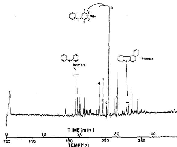
**Figure 1.** FPD chromatogram of the acid-extracted SRC II HD A-3 fraction on a 25% biphenylpolysiloxane stationary phase: temperature program from  $120^\circ\text{C}$  to  $265^\circ\text{C}$  at  $4^\circ\text{C min}^{-1}$ ; hydrogen carrier gas at  $100\text{ cm s}^{-1}$ .
