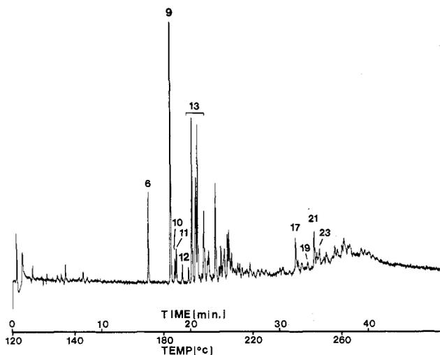
**Figure 3.** Chromatogram of Wyoming Recluse crude oil PAH/PASH fraction on 25% biphenylpolysiloxane column. Conditions are given in Figure 2. Peak numbers refer to compounds listed in Table I.
