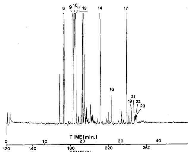
**Figure 2.** Chromatogram of SRC II PAH/PASH fraction on 25% biphenylpolysiloxane column: temperature program from 120 °C to 265 °C at 4 °C min<sup>-1</sup> after an initial 2-min isothermal period; hydrogen carrier gas at 100 cm s<sup>-1</sup>. Peak numbers refer to compounds listed in Table I.
