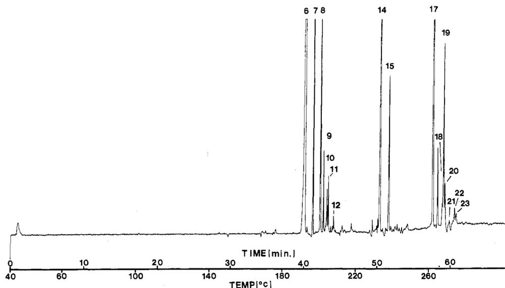
Figure 1. Chromatogram of coal tar on 25% biphenylpolysiloxane column: temperature program from 40 °C to 265 °C at 4 °C min<sup>-1</sup> after an initial 2-min isothermal period; hydrogen carrier gas at 50 cm s<sup>-1</sup>. Peak numbers refer to compounds listed in Table I.
