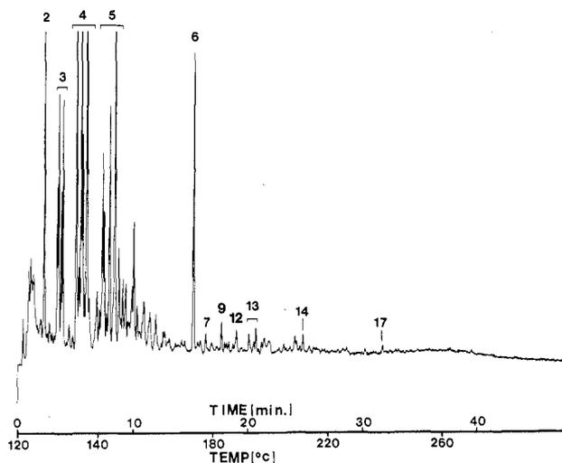
**Figure 4.** Chromatogram of Occidental shale oil PAH/PASH fraction on 25% biphenylpolysiloxane column. Conditions are given in Figure 2. Peak numbers refer to compounds listed in Table I.
