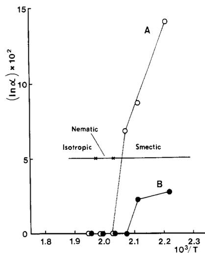
**Figure 2.** Dependence of separation factor ( $\alpha$ ) on column temperature (K) for separation f (A) 3-methyldibenzothiophene/1-methyldibenzothiophene and (B) 2-methyldibenzothiophen/8-methylnaphtho[1,2-*b*]thiophene on PMPS-1,2.
