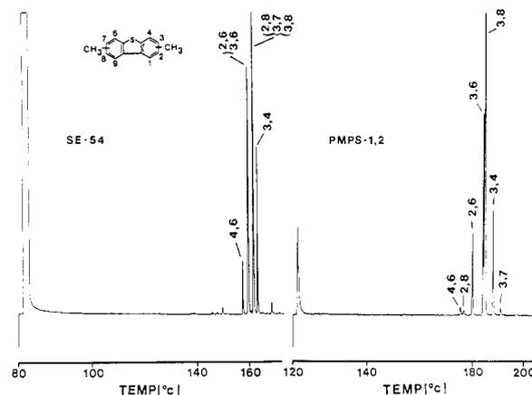
**Figure 3.** Chromatograms of isomeric dimethyldibenzothiophenes on SE-54 (FID) and PMPS-1,2 (FPD). Temperature was programmed from 80 °C (SE-54) and 120 °C (PMPS-1,2) at 4 °C min<sup>-1</sup> with a 2-min initial isothermal period. Hydrogen gas at 100 cm/s was used as the carrier gas.
